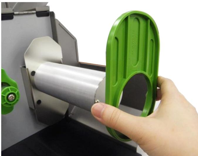
3. Remove the label roll guard from the label spindle.
