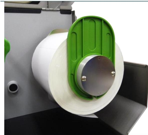
4. Place the roll of media on the label supply spindle and push it to the end of label spindle. Install the label roll guard gently to fit the width of label roll.
