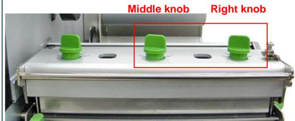
The print head pressure adjustment knob has 5 levels of settings. Clockwise direction adjustment is to increase the print head pressure. Counter Clockwise adjustment can decrease the print head pressure.
