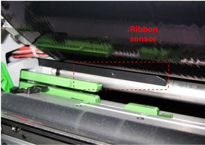
4. Thread the ribbon through the ribbon sensor slot and then through the open space in between print head and platen.
