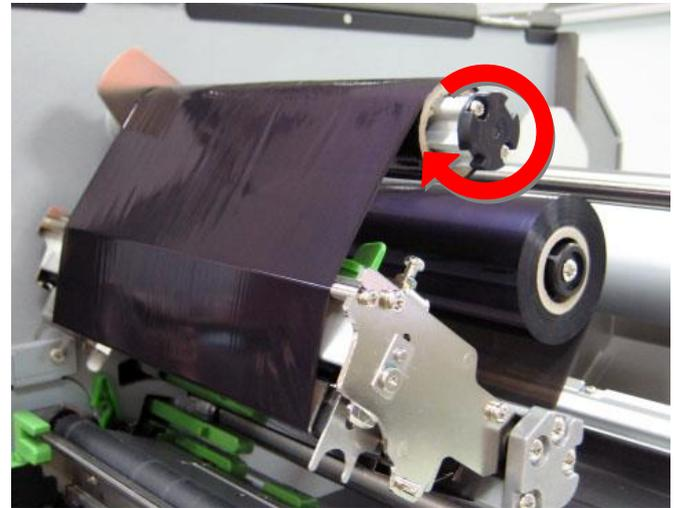
6. Wind the ribbon clockwise about 3~5 circles onto the ribbon rewind spindle until it is smooth and properly stretched.
