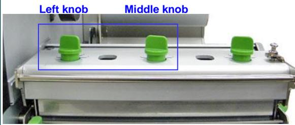
The print head pressure adjustment knob has 5 levels of settings. Clockwise direction adjustment is to increase the print head pressure. Counter Clockwise adjustment can decrease the print head pressure.
