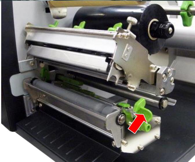
3. Push the print head release lever to open the print head mechanism.
